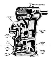
The heart of any sprayer is the pump. The pump used on the Gravely Home'n - garden Sprayer is the nationally famous Myers Du-all Spray pump. This is a double acting, positive displacement pump that delivers ample capacity at all pressures. All working parts are enclosed and fully protected, require a minimum of maintenance.
